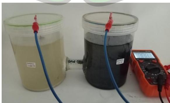
**Gambar 3.4.** Alat reaktor MFC *dual chamber*
