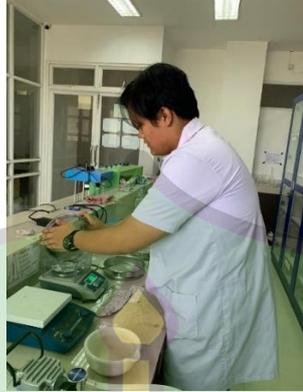
**Gambar 3. 7** Penimbangan Sampel Sedimen Kering
