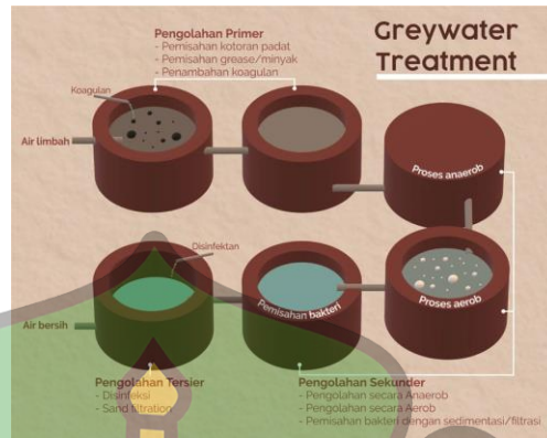
Gambar 4.43 Sistem Greywater Treatment Sumber : https://wastewater.wg.ugm.ac.id/
