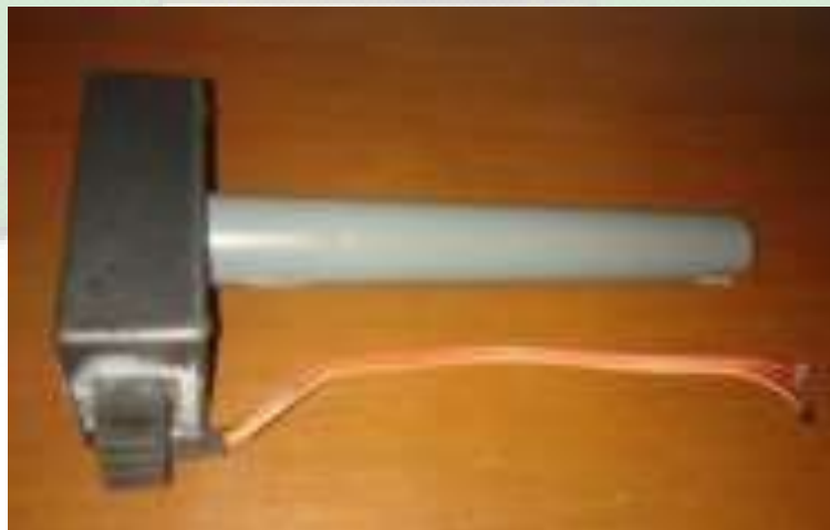
Gambar II.3 Sensor Salinitas Sumber: www.google.com
