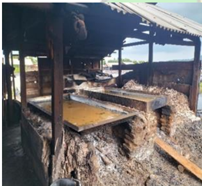
Proses perebusan air garam
